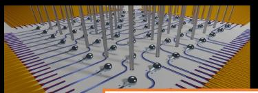
Superconducting Singlephoton detectors (SNSPD)
