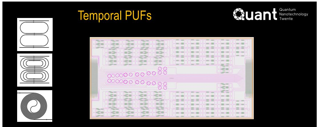
New Chip - PUF designs targeted to give more complexity using a smaller footprint
