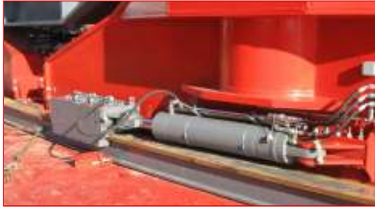
New Design Clamping System Quick-clamping system, at any point on track
