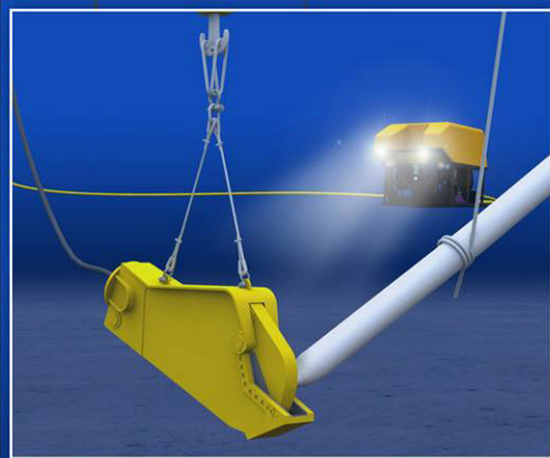
1st Cut Near Seabed Using Shears
