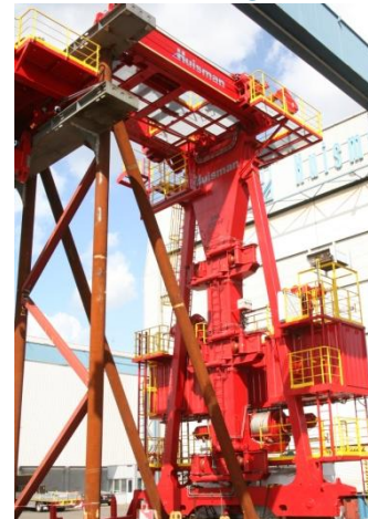
BOP handling crane
