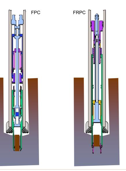
③ Core is cut in undisturbed formation ahead of the drill bit
