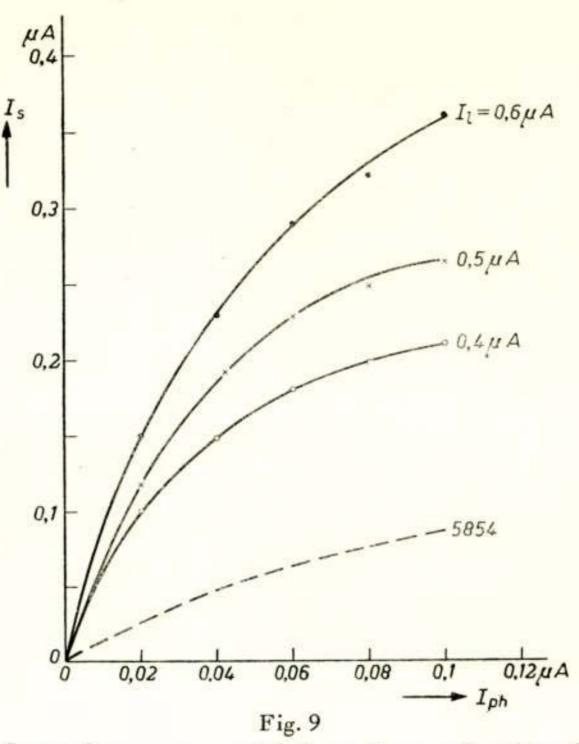
Curve drawn as a solid line:  $I_s$  as a function of  $I_{ph}$  for the "Scenioscope", with the leakage current  $I_l$  through the glass target as a parameter ( $I_l$  measured in darkness). Curve drawn as a dotted line:  $I_s = f(I_{ph})$  for image iconoscope 5854.
