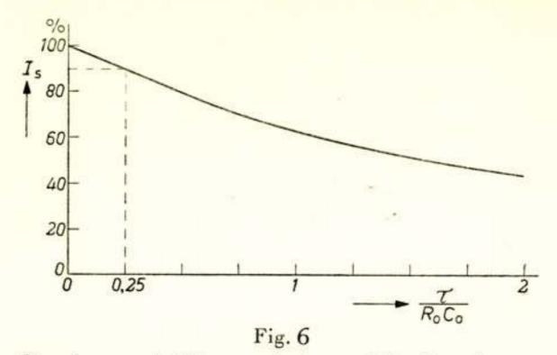
Signal current (Is: on relative scale), plotted as a function of  $\tau/R_oC_o$ , for values of  $R_o$  and  $C_o$  consistent with an  $I_s$  equal to 90% of the maximum value  $(\tau/R_oC_o = 0.25).$
