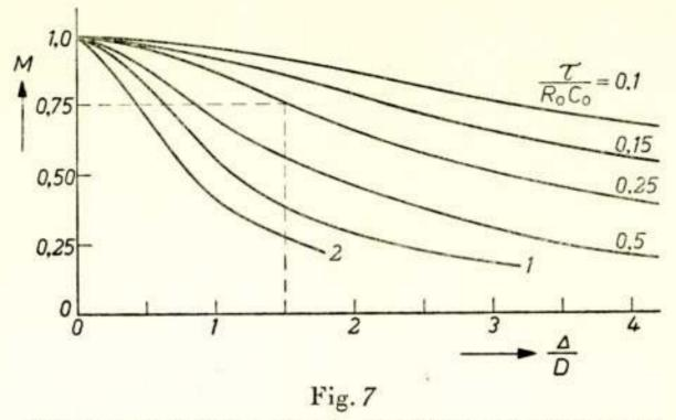
Relative modulation depth M of the potential image on the target, plotted against  $\triangle/D$  ( $\triangle$  = thickness of target, D width of beams in a picture comprising black and white beams), with  $\tau/R_0C_0$  as parameter. For  $\tau/R_0C_0 = 0.25$ ,  $\triangle/D$  must not exceed roughly the value 1.
