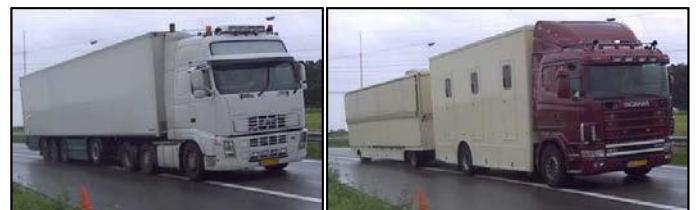
Figure 5. Truck passages at 6 September 2011, truck 1 (left): 32 tons and 6 axles and truck 2 (right): 14.4 tons, 4 axles.
