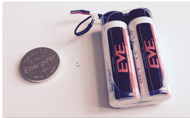
Battery for Mesh sensor (coin cell) versus battery for NB-IoT or Lora sensor (2xAA)
