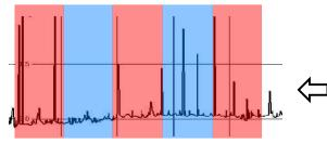
**Frequency domain** Merge the spectra of all frequency blocks Time-domain Sample the frequency interval with high sampling rate
