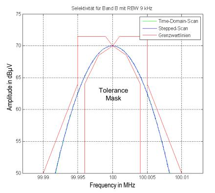
Selectivity for CISPR Band B Measurement BW 9 kHz
