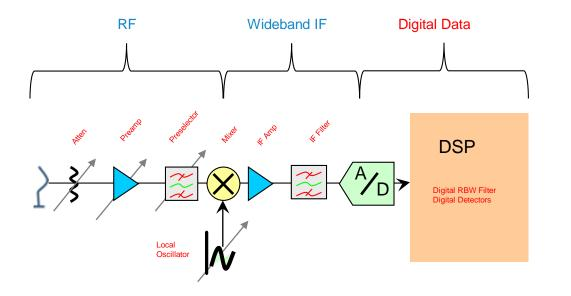
**Wideband** IF into ADC and digital signal processing via dedicated **FPGA** provide for a entire new level of feature / functionality including:
