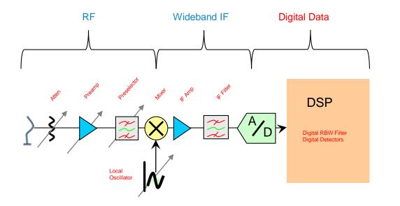
IF into ADC and digital signal processing provide for a entire new level of feature / functionality including:
