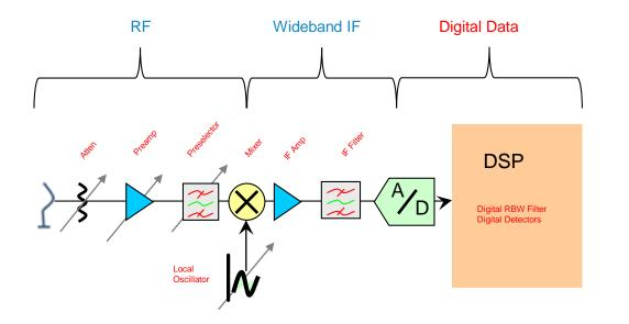
**Wideband** IF into ADC and digital signal processing provide for a entire new level of feature / functionality including:
