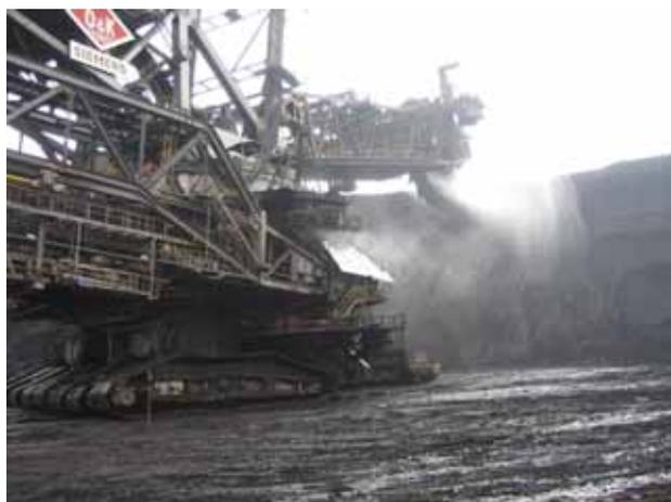
Fig. 1 The 90 m high bucket wheel excavator excavating grey, clayey soil (photo by Arjan Kochx).
