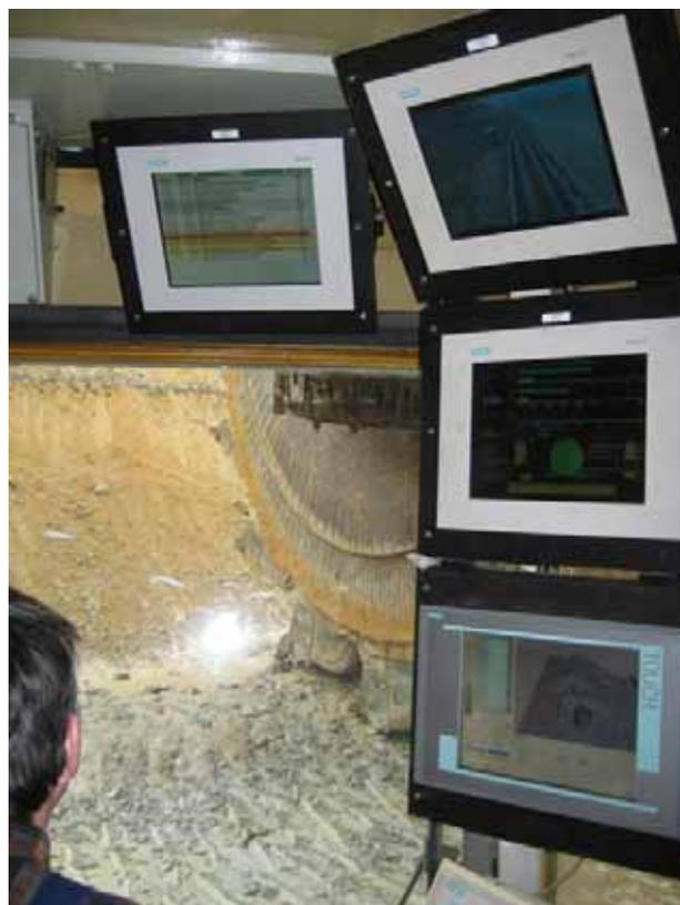
Fig. 2 The IT-system inside the control room of the bucket wheel excavator (photo by Arjan Kochx).
