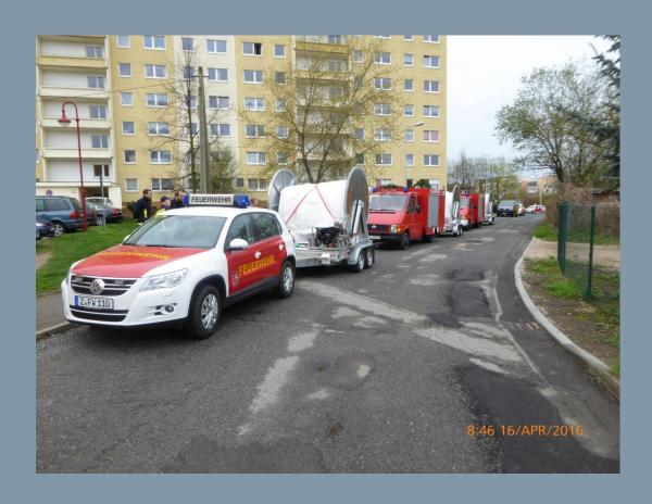
50m MD150-3 on Deichmobil "L". With changeable drums and hydraulic motor. 200m /Std.
