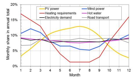
Figure 46: Rough estimate of the monthly distribution (annual total = 100 percent) of solar power calculated for Freiburg [PVGIS], wind power [DEWI], heating requirements based on the heating degree days (VDI Guideline 2067 and DIN 4713), energy requirements for domestic hot water production, electricity demand [AGEB1] and fuel requirements [MWV].
