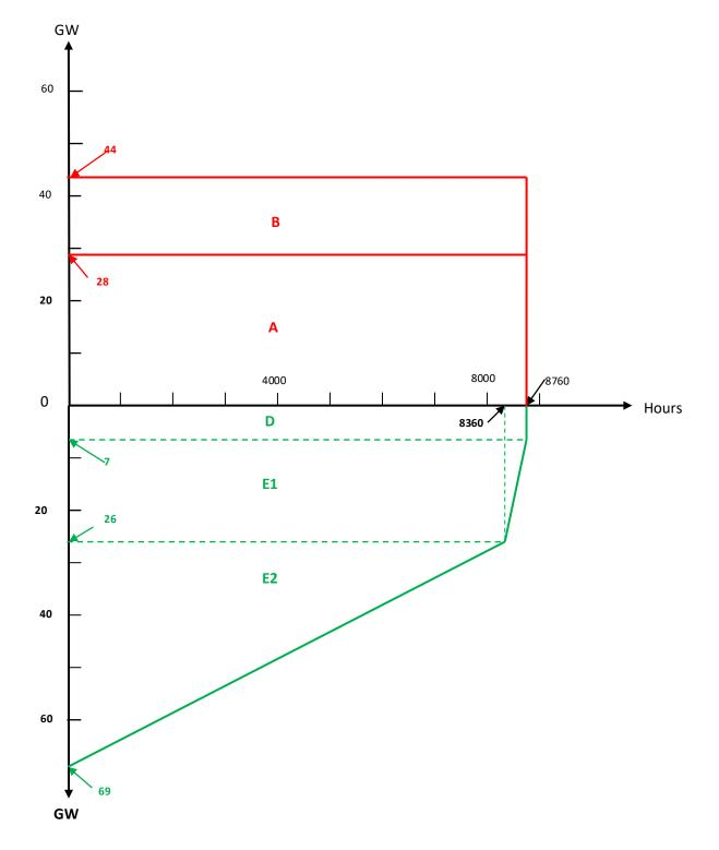
Fig. C3 Actualized Power duration curves, on the negative side of the Power axis the total production; on the positive side the total demand: electricity and H2 plus net losses and backup conversion losses
