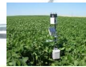
Environmental data – temp. humidity, wind
