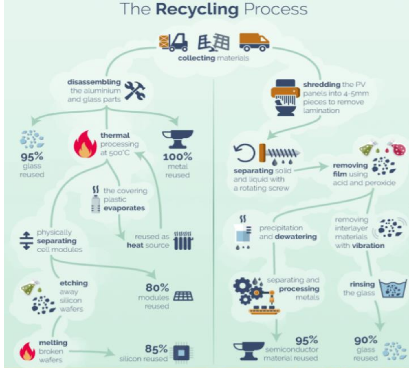
Figuur 1 Het basis recycle proces van zonnepanelen https://www.greenmatch.co.uk/blog/2017/10/the-opportunities-of-solar-panel-recycling
