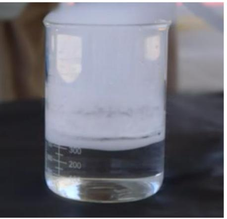
• The volume of LNG is around 1 to 600 of it volume in gas.
